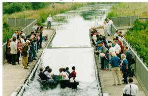
Soliton on the Scott Russell Aqueduct on the Union Canal near Heriot-Watt University, July 1995
